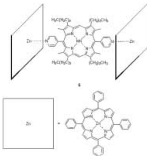
Fig. 9. Schematic representation of a reactive "triad." The central porphyrin is an efficient catalyst for olefin epoxidation. The peripheral porphyrins protect the catalyst from attack by other catalytic centers, thereby extending its lifetime. Squares similarly stabilize catalysts.
