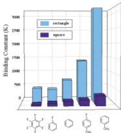
Fig. 8. Binding constants ( $M^{-1}$ ) for several aromatic guest molecules. Rectangle-based materials, which offer good shape complementarity, bind the planar guests much more strongly than do square-derived materials.
