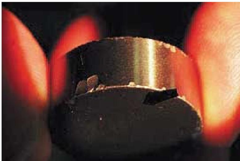
Fig. 2. CVD-prepared thin film (ca. 5  $\mu\text{m}$ )  $\text{V}(\text{TCNE})_x$  magnet on a piece of broken glass being attracted to a  $\text{SmCo}_5$  magnet at room temperature in the air.<sup>5a</sup>
