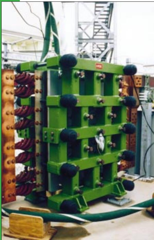
Fig. 1: The first generation three cell electrolyzer stack with an active area of 2.0 m<sup>2</sup>. The electrolyzer was designed by DuPont and DeNora.
