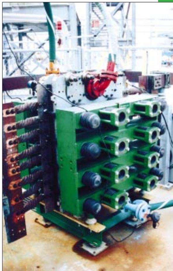
Fig. 2: A second generation three cell prototype electrolyzer with an active area of 2.0 m<sup>2</sup>.
