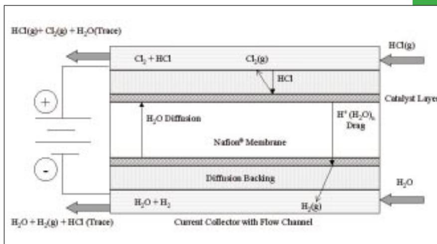
FIG. 5: Schematic of the DuPont Anhydrous HCl electrolyzer and the corresponding electrode and membrane processes.
