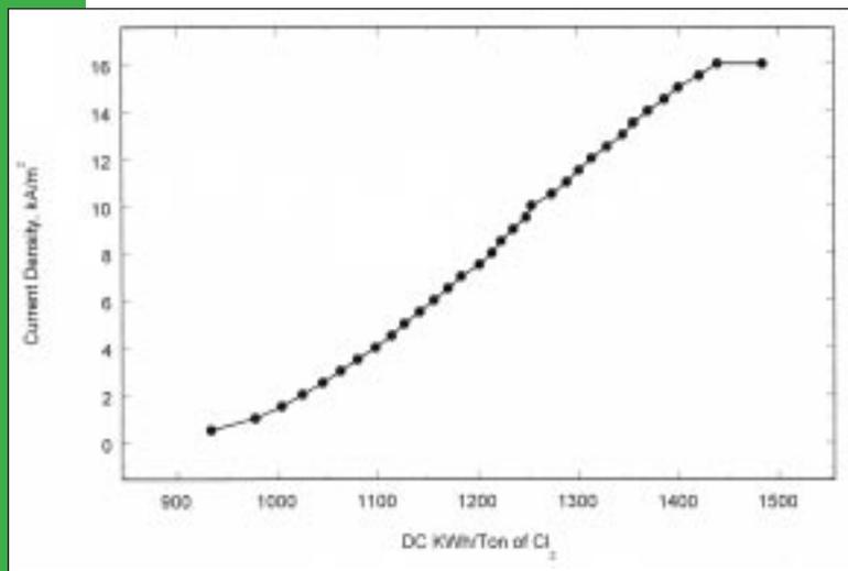
FIG. 4: An experimental polarization curve depicting the relationship between the applied current density and the energy requirements per ton of chlorine.
