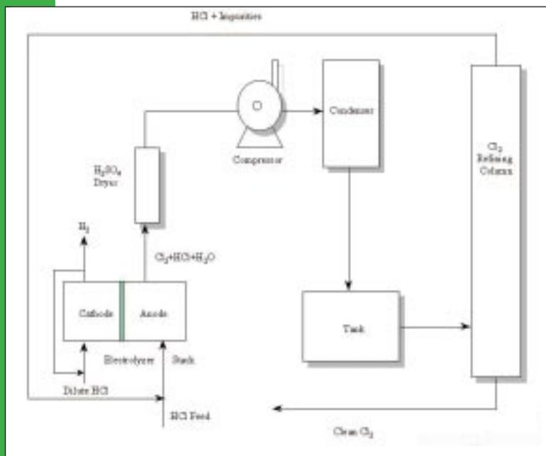
FIG. 3: Process flow sheet for the DuPont Anhydrous HCl Process.
