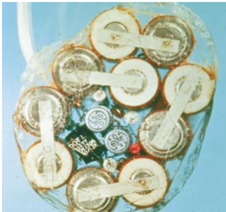
Fig. 1. A very early cardiac pacemaker (ca. 1961), containing two transistors and ten zinc/mercuric oxide primary batteries.
