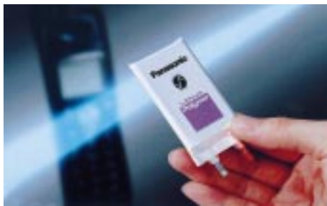
Fig. 2. Li-ion polymer battery. (Photo courtesy of Panasonic.)
