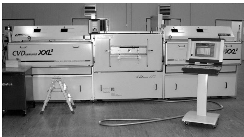
FIG. 2. Largest machine for the production of diamond electrodes (500mm x 1000mm) by hot filament chemical vapour deposition.
