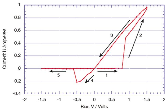
FIG. 7. I-V plots for DMAN-NC<sub>60</sub>, **3** measured in a Au | LB monolayer of **3** | Au cell, with numbers indicating the measuring sequence.<sup>22</sup>
