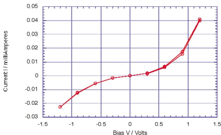
FIG. 8. I-V plots for DMAN-NC<sub>60</sub>, **3** measured in a Au | LB monolayer of **3** | Au cell, in which the current stays small: this should be the current due to **3** and not to the Au filaments.<sup>22</sup>
