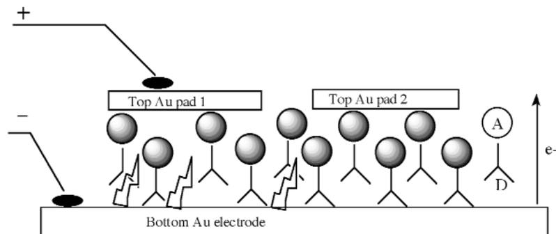
FIG. 6. Schematic of LB monolayer of DMAN-NC<sub>60</sub>, **3** on Au, including top Au pads and Au stalagmites. The direction of preferred electron flow under forward bias is also shown, as an arrow, from the bottom Au electrode to top Au electrode pads.<sup>22</sup>
