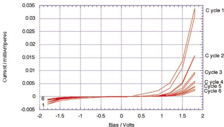
Fig. 5. *I-V* plots for  $(Bu_2N\phi V)_2BuPy^+I$ , **2** measured in a Au | LB monolayer of **2**|Au cell, for six successive cycles of measurement. The rectification ratios are  $RR = 12, 7, 5, 4, 3, 3$ , for cycles 1 through 6, respectively.<sup>21</sup>
