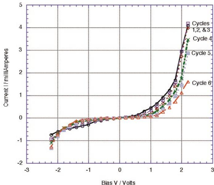
Fig. 4. *I-V* plot for a cell Au|monolayer of  $C_{16}H_{33}Q-3CNQ$ |1|Au, showing the decrease in rectification ratio. At 2.2 V in the first cycle,  $R = 538 \Omega$ ,  $I = 4.09 \text{ mA} = 4.5 \times 10^4$  electrons molecule<sup>-1</sup> s<sup>-1</sup>, and  $RR = 5.39$ . Cycle 1: circles ○; cycle 2: squares □; cycle 3: diamonds ◇; cycle 4: x's X; cycle 5: squares with crosses ⊕; cycle 6: triangles Δ.<sup>18</sup>
