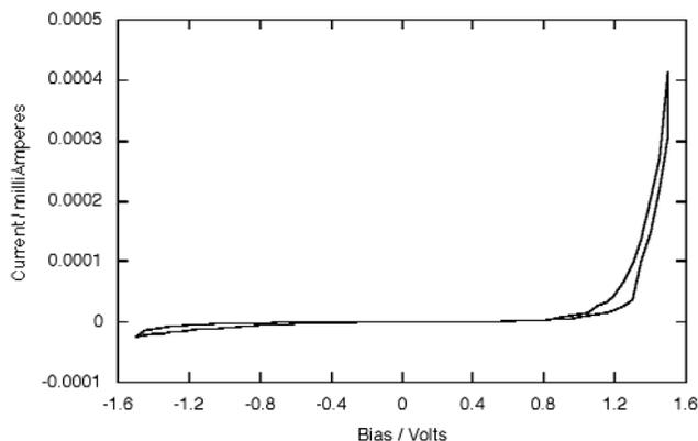
FIG. 3. Plot of the dc current  $I$  vs. the dc applied voltage  $V$  ( $I$ - $V$  plot) through a single monolayer of  $C_{16}H_{33}Q-3CNQ$ , **1** sandwiched between Al electrodes (top Al pad area  $4.5 \text{ mm}^2$ , thickness  $100 \text{ nm}$ ), using Ga/In eutectic and Au wires. The dc voltage is swept at a rate of  $10 \text{ mV s}^{-1}$ .<sup>14</sup>
