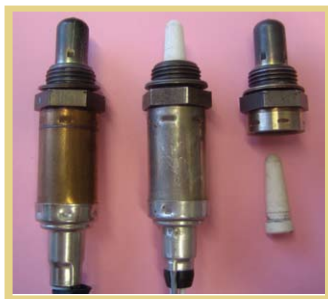
Fig. 3. Lambda (λ) probe as originally developed by Bosch using doped zirconia as described by Kiukkola and Wagner. 1
