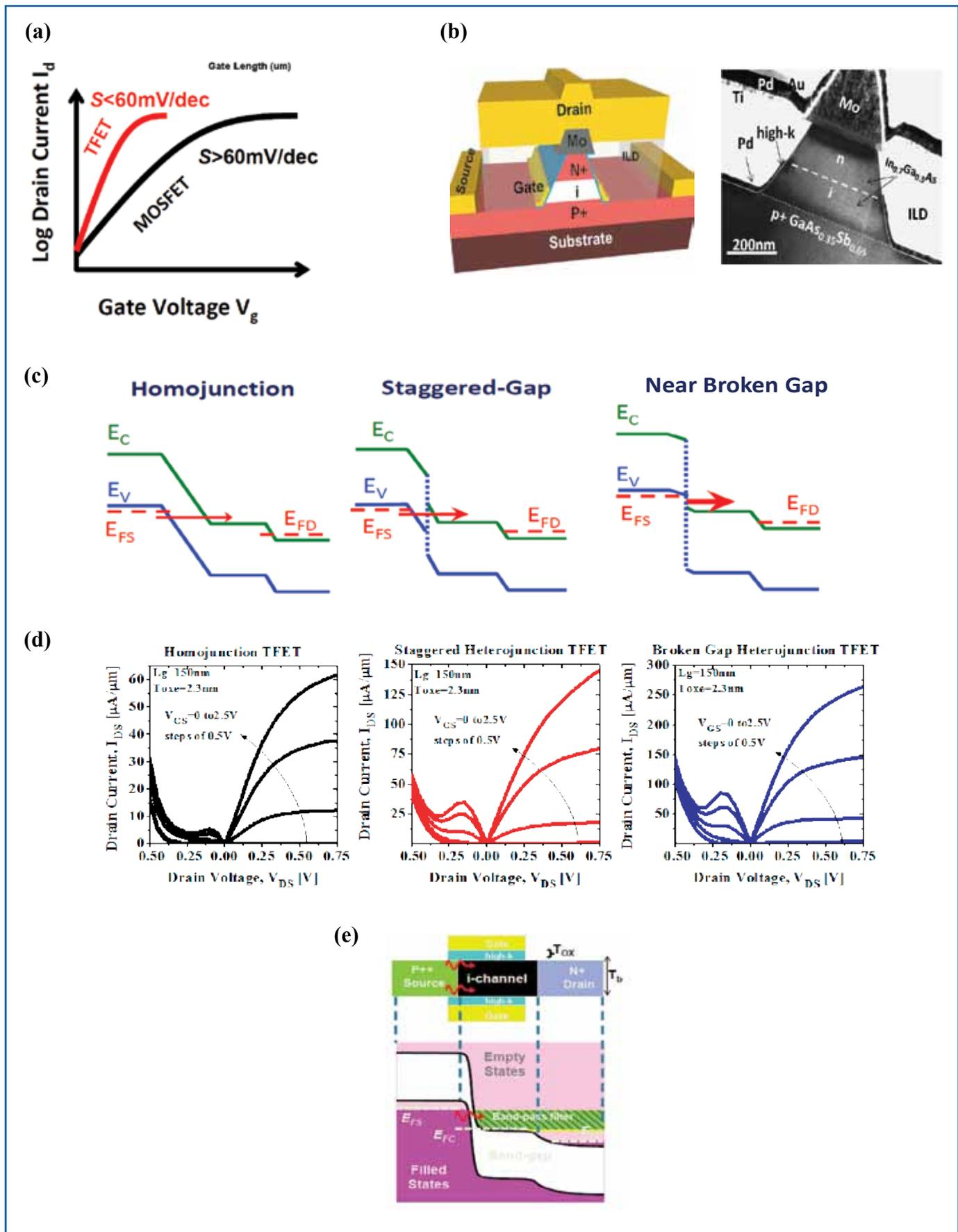
FIG. 5. (a) Energy band diagram of Tunnel FET (TFET) showing steep switching transfer characteristics. (b) Schematic and cross-section of vertical 3D nanopillar TFET. (c) Schematic band diagram of homojunction, staggered gap and near broken gap heterojunction TFETs. (d) Experimental output characteristics of homojunction, staggered-gap and nearly broken gap heterojunction TFETs showing significant increase in drive current.<sup>15</sup> (e) Energy band diagram of Tunnel FET.
