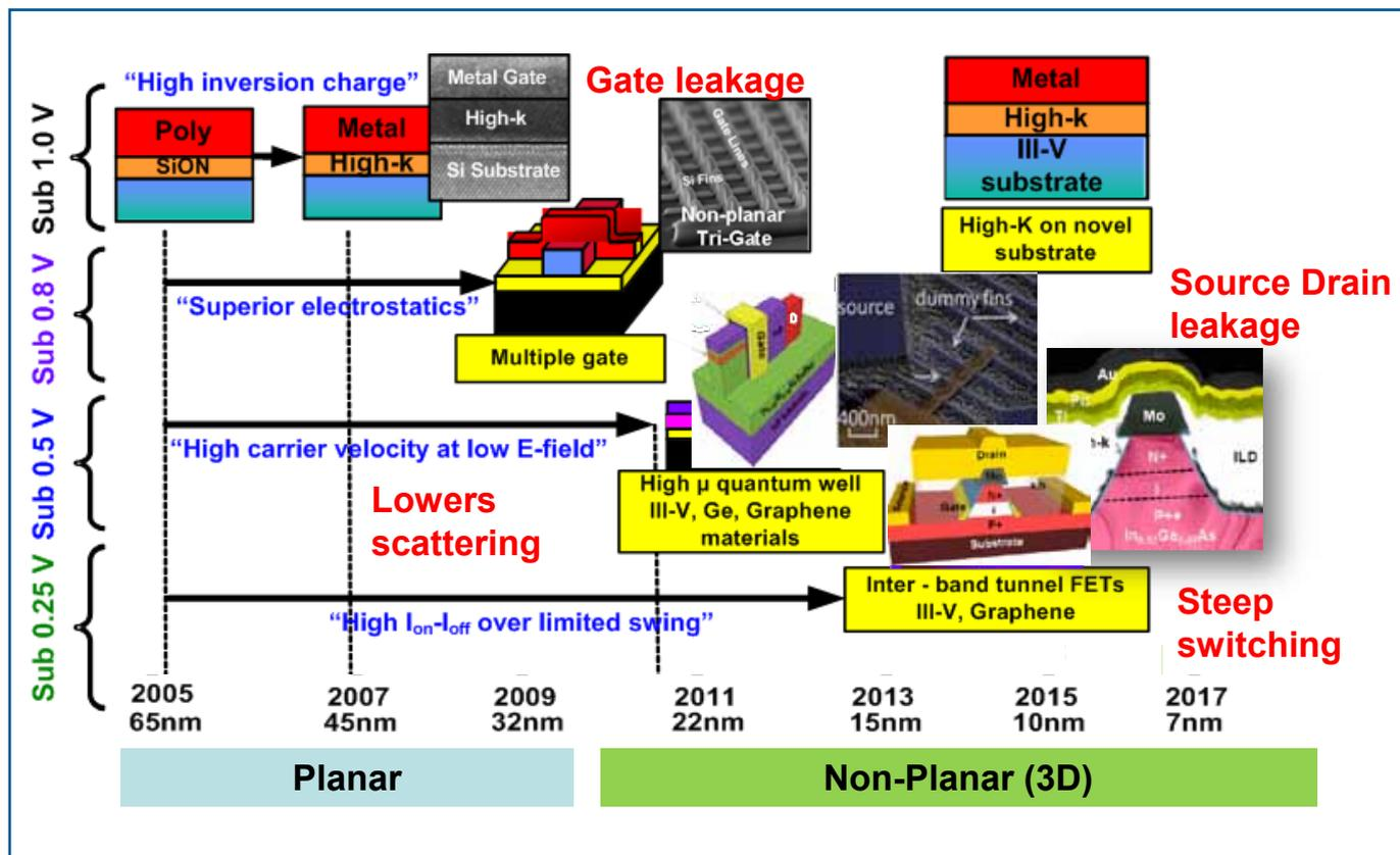
FIG. 1. Trend in state-of-the-art high performance (HP) CMOS transistor innovation. Transformative changes in materials (high-k dielectric, Ge, III-V channel) and the transistor architecture (3D, Tunnel FET) being implemented and explored to maintain historical rate of performance, density and power scaling.
