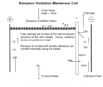
Fig. 1. Sampson Oxidation Membrane Cell. Depicts bromine production although chlorine dioxide is generated in a similar manner. Figure courtesy of Halox Technologies Corporation (Bridgeport, CT).
