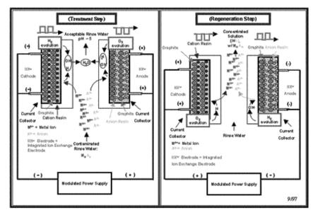
FiG. 3. In-process recycling system which integrates electrowinning and ion-exchange into one system, combining the benefits of both. Figure courtesy of Faraday Technology, Inc. (Clayton, Ohio).
