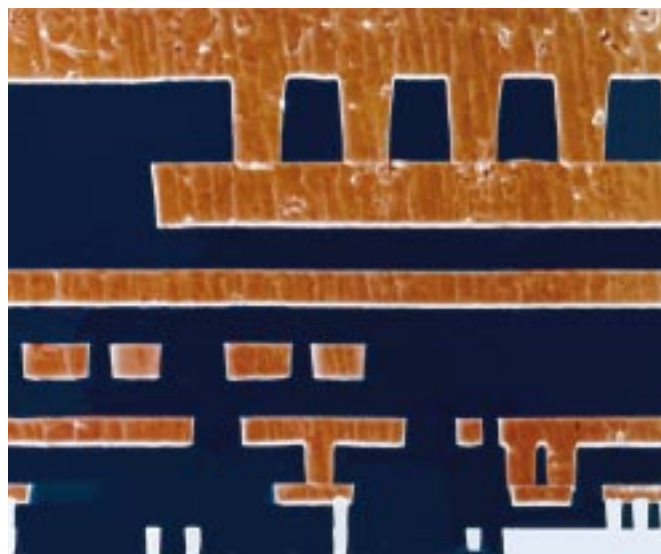
Fig. 1. Cross section of a 6-level copper wiring structure fabricated by IBM showing wiring hierarchy.
