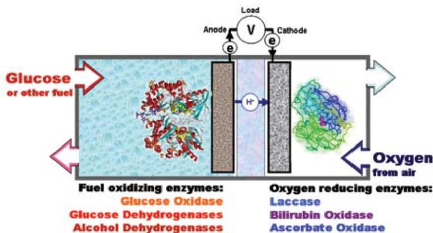
**FIG. 1.** Generalized schematics of an enzyme biofuel cell consisting of an anode, catalyzed by oxidases suitable for conversion of fuels of choice or a complex of such enzymes for a complete oxidation of biofuels. The cathode usually features an oxidoreductase that uses molecular oxygen as the ultimate electron acceptor and catalyzes reduction to water in neutral or slightly acidic media.
