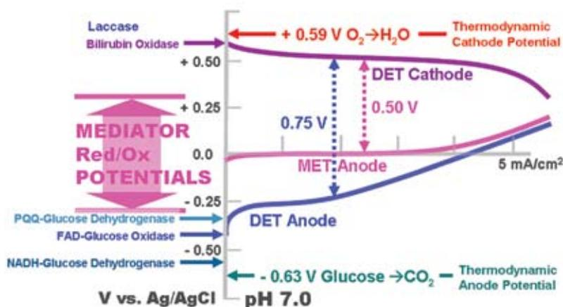
**FIG. 2.** Principles of biofuel cell design indicating the maximum oxidation potentials for glucose and the corresponding thermodynamic potential for oxygen reduction at neutral pH. Redox potentials of several enzymes and their corresponding co-factors are shown along with the potential "zone" containing the redox potentials of the usual mediators. Polarization curves depict typical current performances for direct and mediated electron transfer in biofuel cell electrodes.
