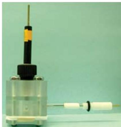
FIG. 3. Standardized stack cell design for the biofuel cell.
