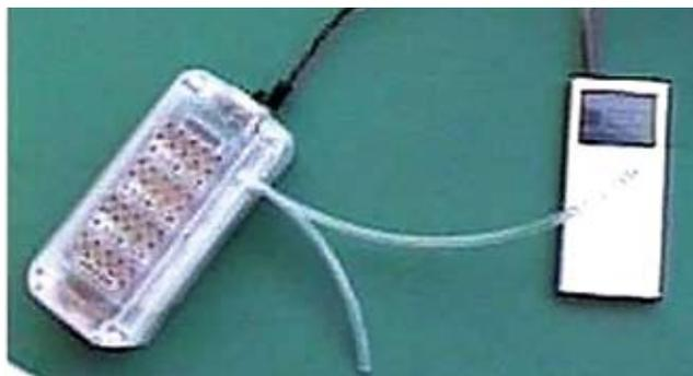
FIG. 4. Ethanol/air biofuel cell stack. This prototype, developed by Akermin, Inc. in 2006, powers an iPod. Photograph courtesy of Akermin, Inc.
