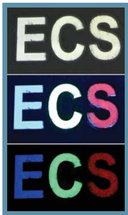
FIG. 2. The persistent luminescence behavior of the blue emitting Sr 2 MgSi 2 O 7 :Eu 2+ ,Dy 3+ (E), green emitting SrAl 2 O 4 :Eu 2+ ,Dy 3+ (C) and red emitting Y 2 O 2 S:Eu 3+ ,Mg 2+ ,Ti IV (S) phosphors in day light, under UV excitation, and in dark.
