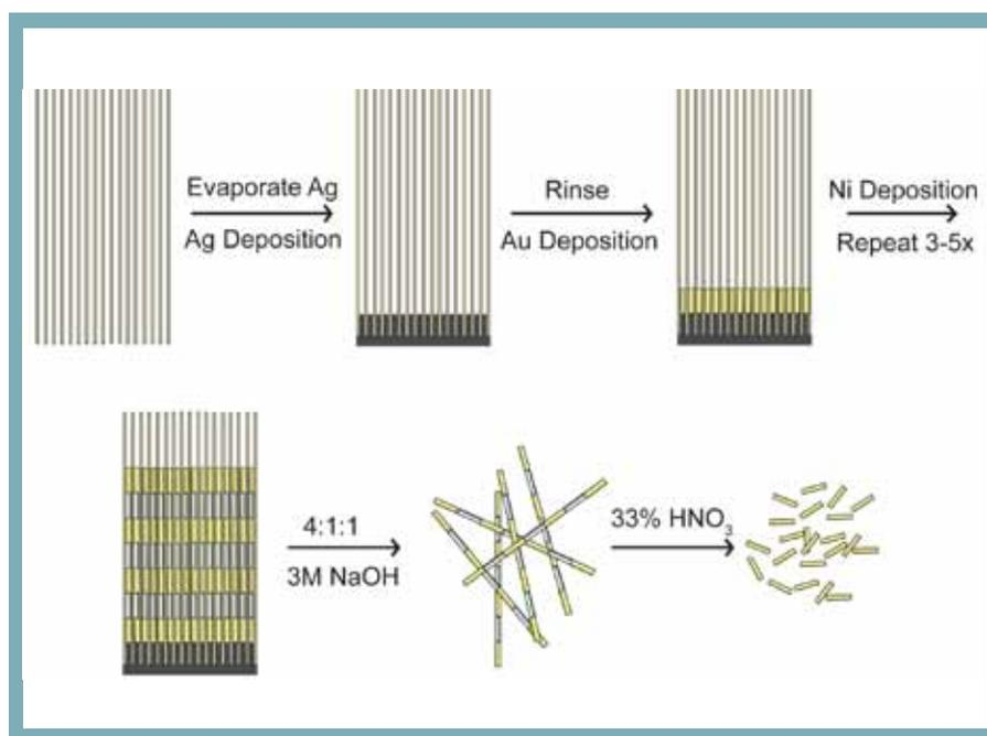
FIG. 1: The template-directed electrochemical growth of metal nanorods.
