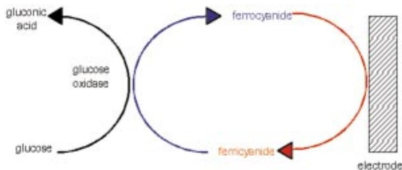
Fig. 3. The reaction sequence for glucose measurement on the Accu-Chek Advantage sensor.
