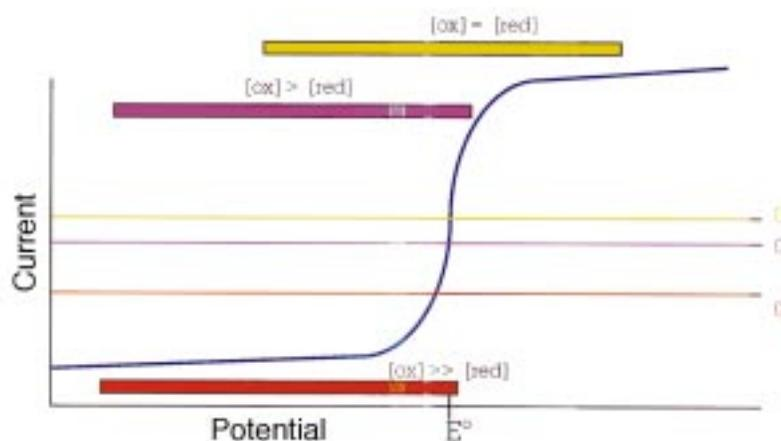
Fig. 6. The general principle of the electrochemical mechanism of Advantage<sup>®</sup> sensors is illustrated. The yellow bar shows the 150 millivolt potential window with equal oxidized and reduced mediator concentrations (a situation we must never reach in the sensor); the purple bar shows the potential window with slightly more oxidized than reduced mediator (high glucose concentrations), and the red bar shows the situation at oxidized >> reduced (low glucose.)
