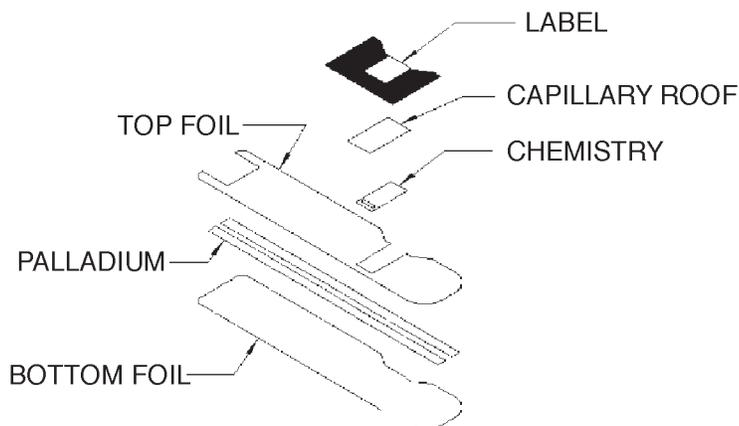
Fig. 2. An exploded view of the Accu-Chek™ Comfort Curve™ biosensor test strip.
