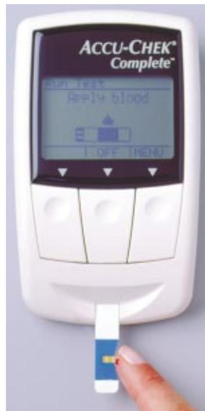
Fig. 1. The Accu-Chek™ Comfort Curve™ biosensor test strip in the Accu-Chek™ Complete™ test device.
