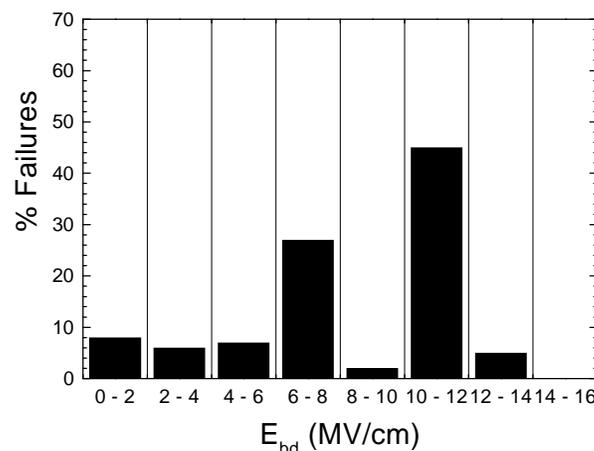
**Figure 2** – Typical dielectric breakdown field ( $E_{bd}$ ) distribution (100 capacitors – gate area of 10<sup>-2</sup> cm<sup>2</sup>) for sample g-90 (cleaning recipe g and oxidation time of 90 minutes).
