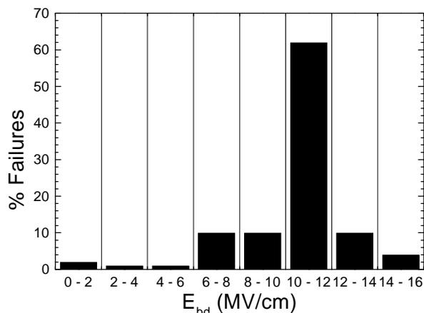
**Figure 1** – Typical dielectric breakdown field ( $E_{bd}$ ) distribution (100 capacitors – gate area of 10<sup>-2</sup> cm<sup>2</sup>) for sample f-90 (cleaning recipe f and oxidation time of 90 minutes).
