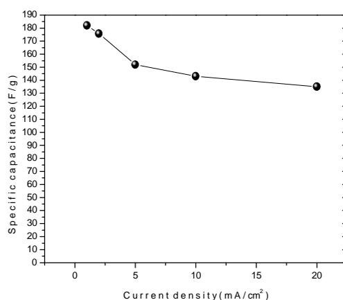
**Figure 2.** Specific capacitances of unit-cell on current densities.
