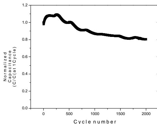
**Figure 3.** Cycle-life performance at 10 mA/cm<sup>2</sup> of current density.
