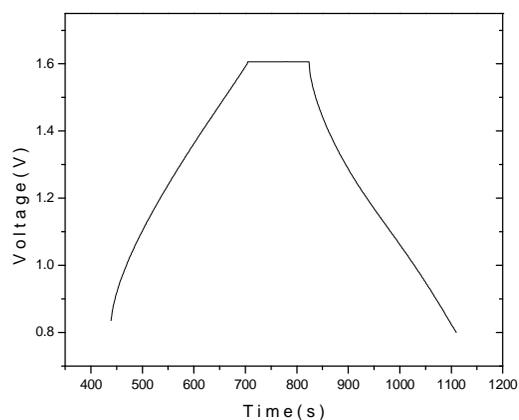
**Figure 1.** Charge-discharge cycle at 10 mA/cm<sup>2</sup> of current density.
