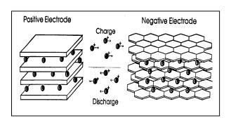
Figure 1. Depiction of the Charge-Discharge Operation of Li-Ion Cells.
