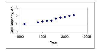
Figure 3. Increase in Capacity of ICR18650 Cells with Time
