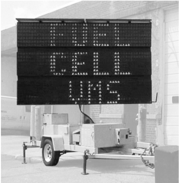
Fig. 1. Solar-Powered Variable Message Sign With Two 50W PEM Fuel Cells For Backup Power
