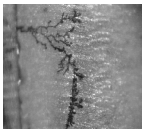
Fig. 1. Typical Dendrite in an Al 2 O 3 substrate
