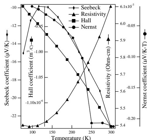
Figure 1. Transport data for GaAs<sub>1-x</sub>N<sub>x</sub> (0.4% N)
