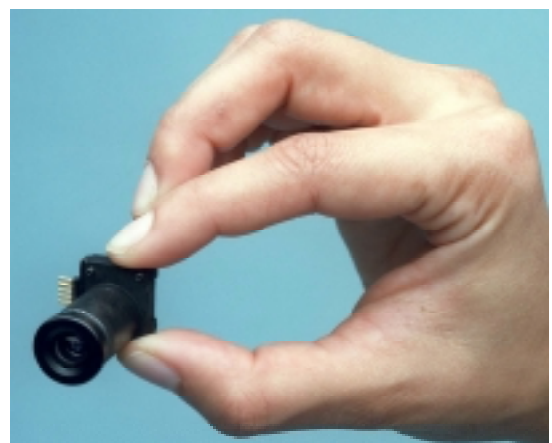
Fig.3 Miniature digital one-chip camera
