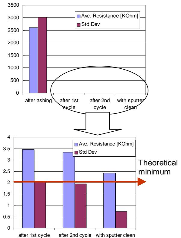
Figure 3 Contact resistance measured after each process steps. Use of oxygen plasma-HF cleaning integrated process reduced contact resistance close to the theoretical minimum value and pre-sputter cleaning reduced standard deviation of contact resistance distribution
