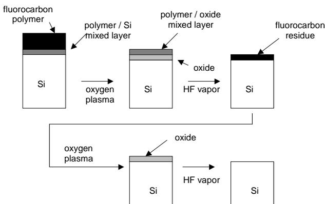
Figure 1 A schematic diagram of contaminated films and the proposed removal procedure.
