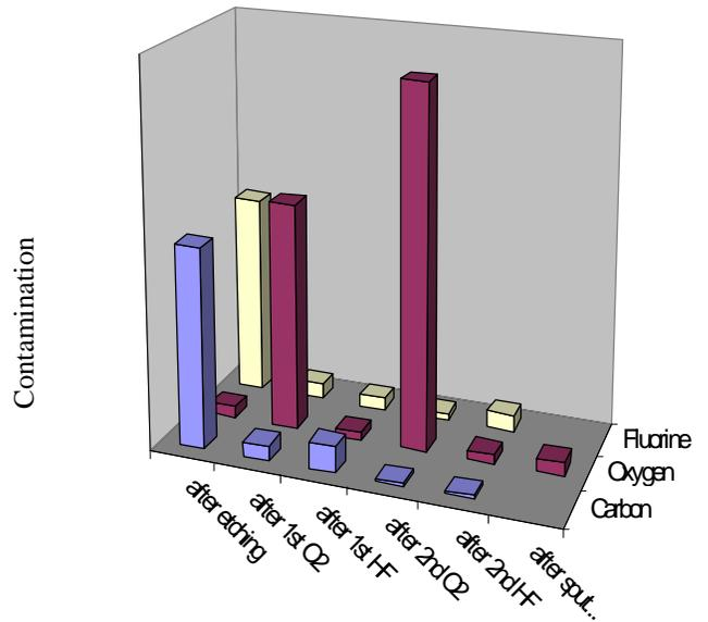
Figure 2 A histogram of contamination measured after each process steps. The integrated cleaning cleaned out the contaminated surface leaving less than half monolayer of contamination, which was subsequently removed by pre-sputter cleaning. Trace amount of oxygen left on the surface after sputter cleaning is captured during sample transfer
