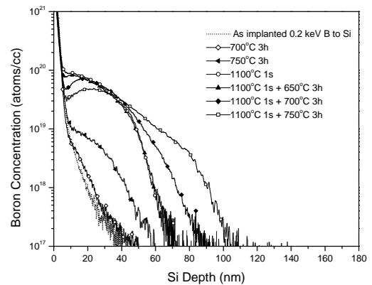
Figure 1. SIMS profile of boron in boron-implanted and annealed samples. After 0.2 keV boron implantation, half of the samples was spike annealed at 1100 °C for 1 sec, followed by furnace annealing at 600 °C, 700 °C or 750 °C for 3 h, respectively. Half of the samples without spike annealing was annealed at 700 °C or 750 °C for comparison.
