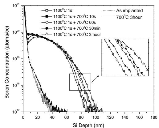
Figure 2. SIMS profiles of boron in as-implanted and annealed samples. After 0.2 keV boron implantation, samples was spike annealed at 1100 °C for 1 sec, followed by furnace annealing at 700 °C for 10 s, 60 s, 30 m, and 3 h, respectively. Sample annealed at 700 °C for 3 h without spike annealing was included for comparison.
