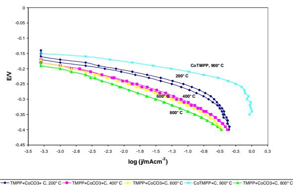
Fig. 1 - Polarization curves in O<sub>2</sub>-saturated alkaline solution of CoCO<sub>3</sub> + TMPP pyrolyzed at various temperatures, then mixed with carbon.
