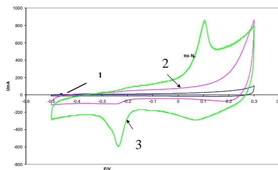
Fig. 2 - Cyclic voltammetry in N<sub>2</sub>-saturated alkaline solution. 1) CoTMPP pyrolyzed at 900°C; 2) CoCO<sub>3</sub> + TMPP + C at 400°C; 3) Same as 2 but at 800°C.
