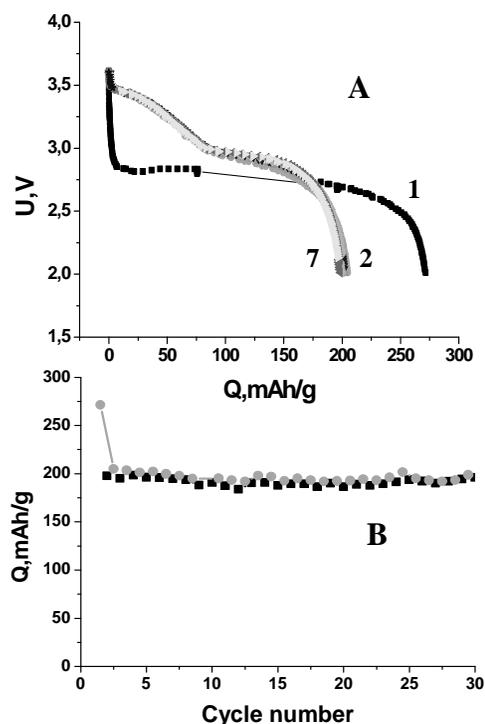
**Fig. 2** Charge-discharge cathode characteristics of  $\text{Li-MnO}_2$  cell (A) and the change of specific discharge capacity at cycling (B).
