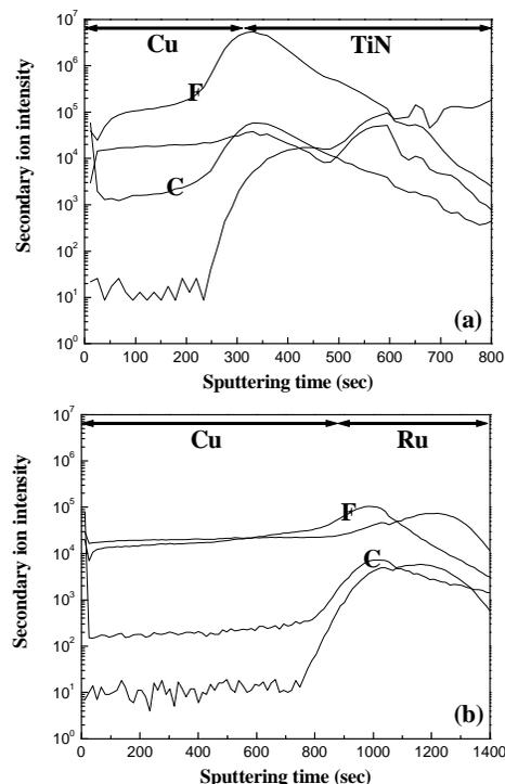
Fig. 2. The depth profiles of copper films (a) on TiN, (b) on ruthenium substrates.
