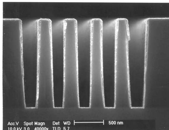
Fig. 1. Cross sectional SEM image showing the excellent step coverage of an ALD ruthenium.
