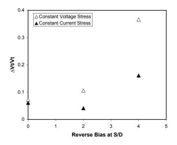
Fig. 1.  $\Delta V_t / V_t$  due to voltage and current stress as a function of reverse biased voltage for substrate injection case.
