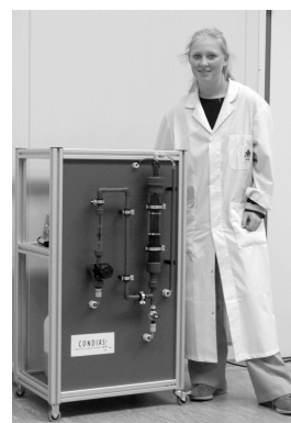
Figure 3: EAOP pilot cell using DiaChem® electrodes. Cell design and fabrication by G.E.R.U.S. mbH, Berlin
