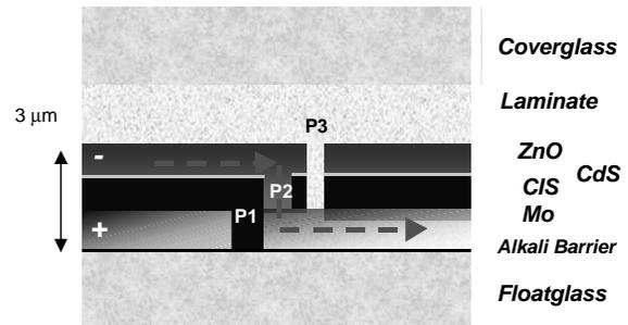
Fig. 2. Schematic cross section through integrated series connection in CIGSSe modules
