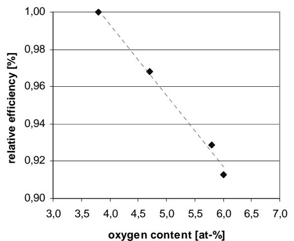
Fig. 4. Direct correlation of oxygen content in CdS film and cell efficiency
