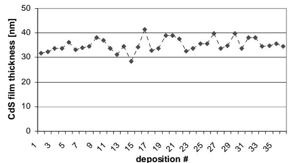
Fig. 3. CdS film thickness data reached in repeated CBD processes
