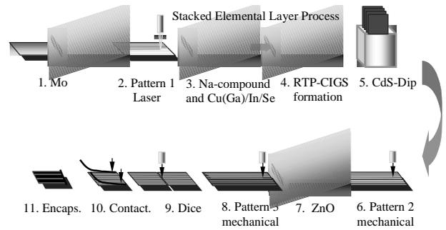
Fig. 1. Process scheme for CIGSSe-modules with monolithic integration of series connected cells
