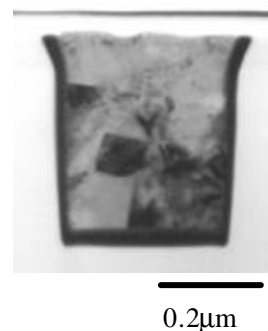
Fig.4. The cross-sectional TEM image of damascene Cu interconnection formed by electroless plating of Cu initiated by displacement reaction on TaN.
