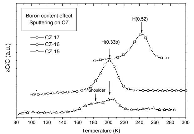
Fig.3: The defects created by sputtering result from reactions of intrinsic defects with impurities hence the DLTS signatures depend on the material type, hydrogen contamination etc. Here we show the DLTS spectra from sputter damaged CZ silicon of different boron concentrations  $5 \times 10^{17}$  (top),  $6 \times 10^{16}$  and  $5 \times 10^{15} \text{ cm}^{-3}$  (bottom)
