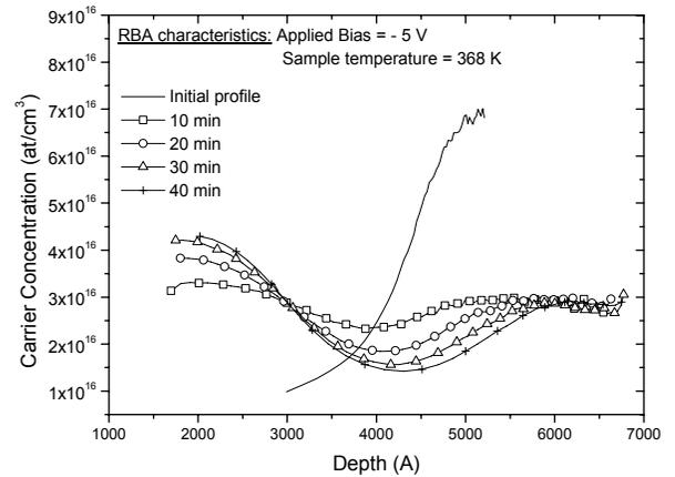
Fig. 1: Free carrier concentration profiles derived from CV measurements on a thin MBE silicon layer. The apparent profile changes after low temperature anneals under reverse bias. The effect is due to inadvertent hydrogen contamination during cleaning.
