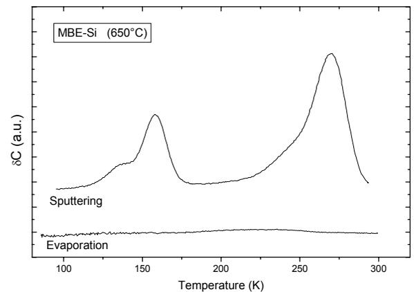
Fig. 2: Comparison of DLTS spectra taken from the near surface region of MBE grown silicon on which titanium Schottky barriers have been deposited by sputtering (top) and by thermal evaporation (bottom).
