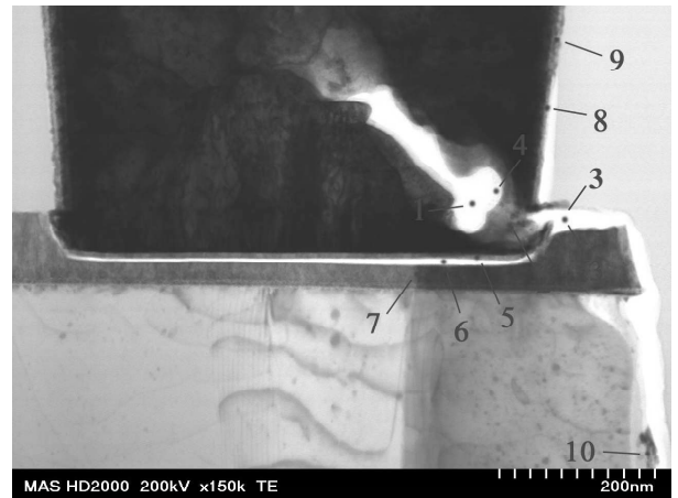
Figure 2: TEM analysis of hollow via. EDX (not shown) shows signs of carbon at locations 3 and 10, top and sidewall of metal line, respectively
