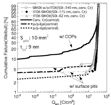
Fig.2 Weibull plot of  $Q_{BD}$  characteristics of 9-nm gate oxide on ITOX-SIMOX wafers fabricated on conventional Cz Si wafers.
