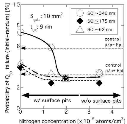
Fig.3 Relation between probability of  $Q_{BD}$  failure (initial + random) on ITOX-SIMOX and nitrogen concentration in the starting material.
