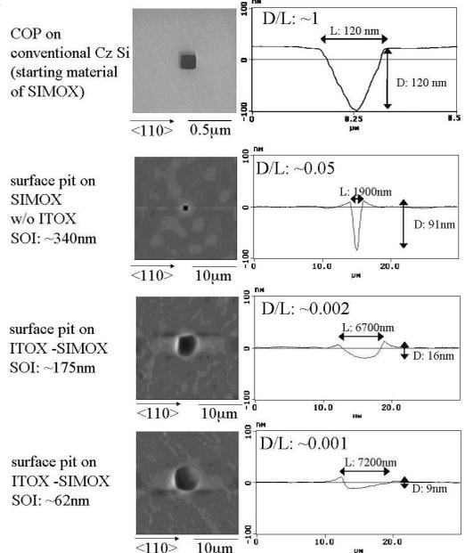
Fig.1 Typical AFM view of surface pits on ITOX-SIMOX fabricated on the conventional Cz Si together with that of COP on the unprocessed Cz Si wafer as comparison.
