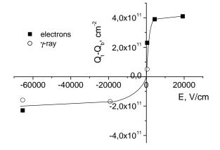
Fig.1. Difference between charges at the bonded interface  $(Q_b)$  and interface formed during thermal oxidation thermal  $(Q_t)$  in SOI as a function of the internal field strength (E) for dose of irradiation of  $3x10^4$  rad.
