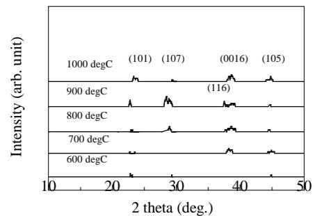
Fig.3. XRD patterns of 0.80Ta<sub>2</sub>O<sub>5</sub>-0.20SiO<sub>2</sub> thin films annealed at various RTA temperatures.
