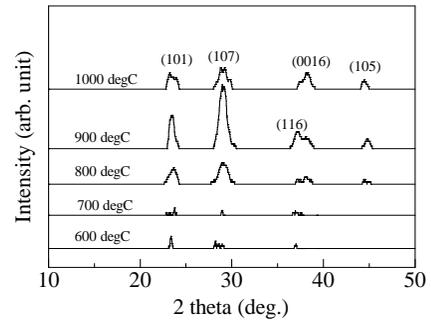
Fig.2. XRD patterns of Ta<sub>2</sub>O<sub>5</sub> thin films annealed at various RTA temperatures.
