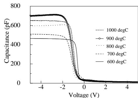
Fig.4. The C-V characteristics of 0.80Ta<sub>2</sub>O<sub>5</sub>-0.20SiO<sub>2</sub>-based MIS structures at various RTA temperatures.
