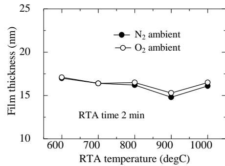
Fig.1. Effect of RTA temperature on the (1-x)Ta<sub>2</sub>O<sub>5</sub>-xSiO<sub>2</sub> (x=0.20) thickness at different ambient.
