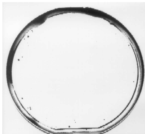
Fig. 2. Scanning Acoustic Microscope image of double bonded SSOI wafer structure
