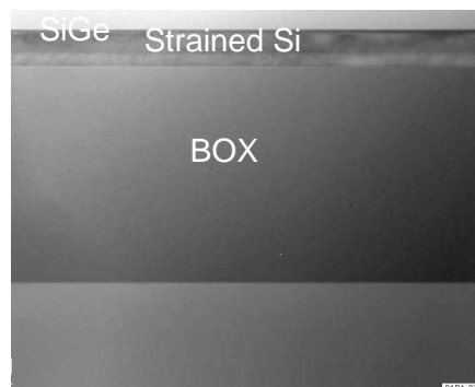
Figure 1 : Strained Silicon On insulator structure based on SiGe layer transfer.
