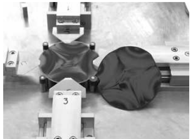
Figure 2: Cleaving device with completely debonded wafer pair. The wafers bonded under hydrophilic condition and annealed at 1100° C for 5 h.
