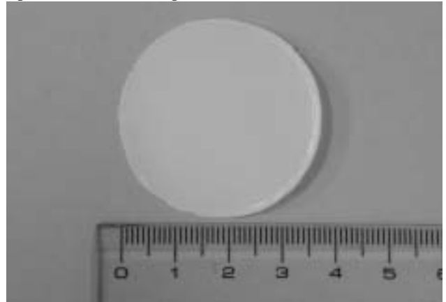
Fig. 1 Photograph of silica membrane prepared from polystyrene beads and colloidal silica after heating at 900°C 1 h.
