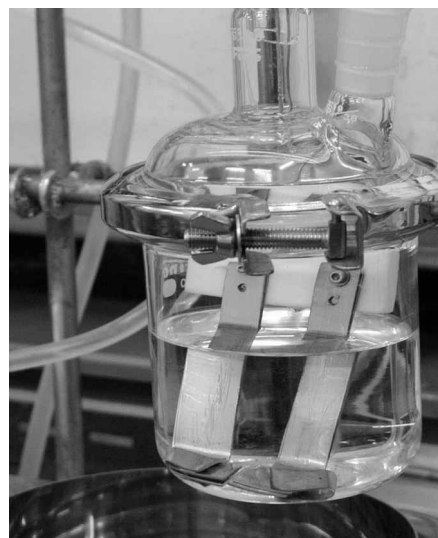
Fig. 1 Chamber for synthesis of carbon nanotubes in organic liquid
