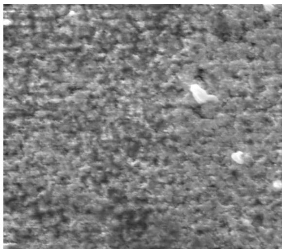
Fig. 2. SEM image (5000 X) of a electrodeposited PbTe film on PSL during 30 min at a current density of 0.14 \text{mA}/\text{cm}^2 .
