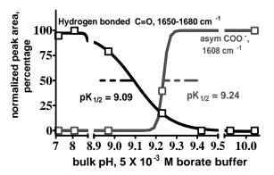
measurements and report here our findings. The apparent  $pK_{1/2}$  (ie., the bulk pH- value at which 50% of the mercaptoundecanoic acid is ionized) is seem in Figure to be  $9.1\pm0.1$ . Applying potential at pH = 0.1 (in the absence of water) has also changed the extent of the ionization of the SAM. Significance of these results are discussed.
