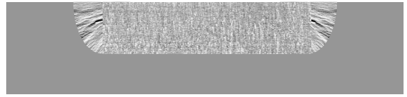
Figure 1. SEM cross-sectional view of a porous Si nanostructure formed by electrochemical anodization of bulk monocrystalline Si substrate.
