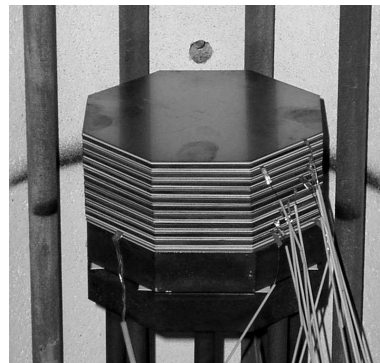
Figure 2. External view of a 10-cell stack with 5 cm x 5 cm single-cells. Steady-state polarization of the electrode at 1073 K.
