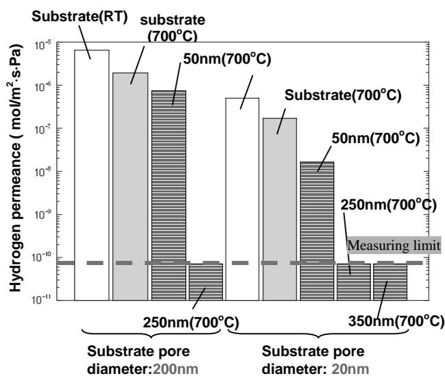
Fig. 2. Gas permeance of the deposited YSZ thin films. (Numbers on graph indicate film thickness and heat temperature)
