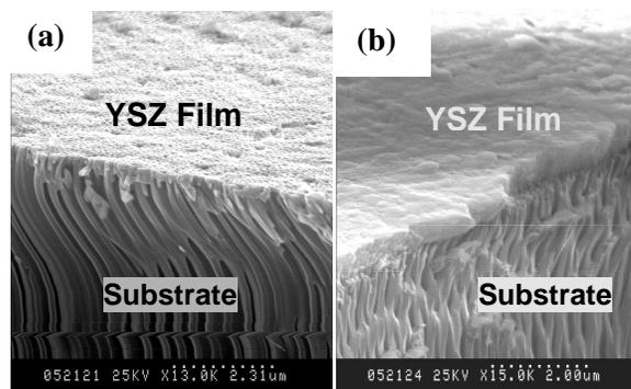
Fig. 1. SEM images of YSZ thin films with a thickness of (a)30nm and (b)250nm on nanoporous anodic alumina substrates.
