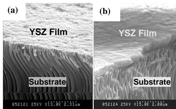
Fig. 1. SEM images of YSZ thin films with a thickness of (a)30nm and (b)250nm on nanoporous anodic alumina substrates.
