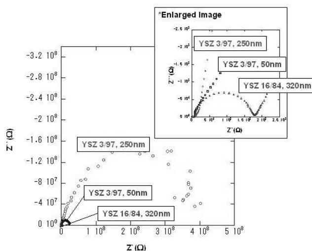
Fig. 3. Nyquist plots of YSZ thin film with different composition.
