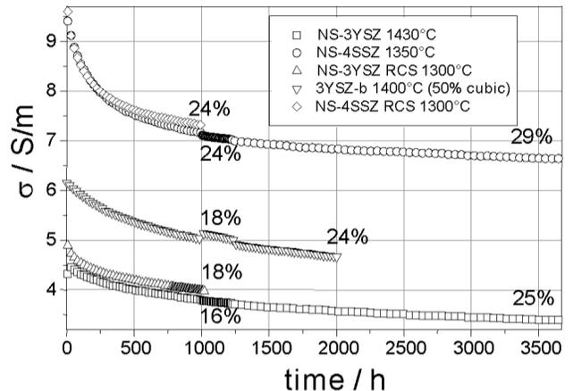
Fig. 2: Electrical conductivity decrease of 3YSZ and 4SSZ electrolyte tapes sintered with various temperature profiles.
