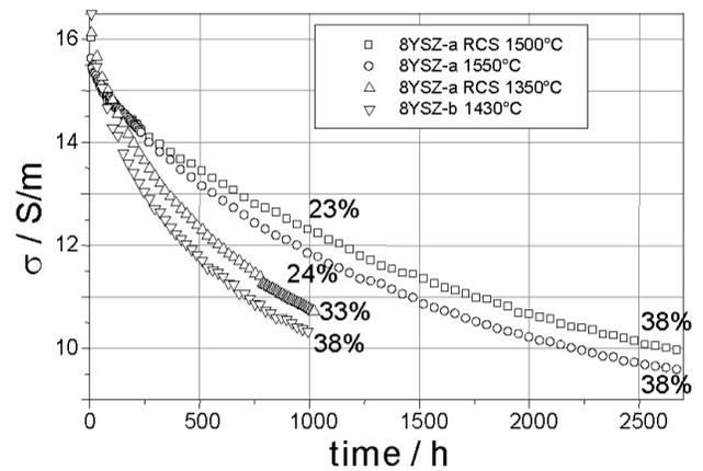
Fig. 1: Electrical conductivity decrease of 8YSZ electrolyte tapes sintered with various temperature profiles.
