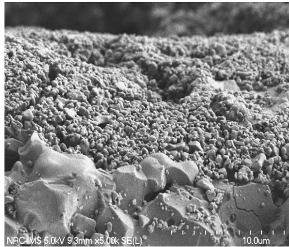
Figure 1 – SEM micrograph of LSGM electrolyte with 10% Co doped \text{La}_2\text{NiO}_{4+\delta} cathode layer.
