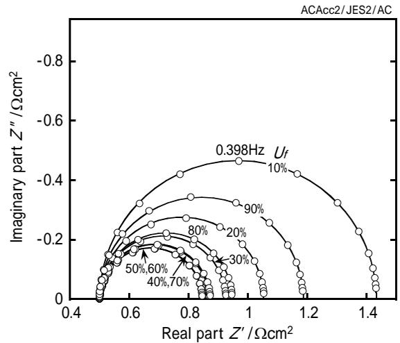
Fig.2 Simulated behavior of ac impedance at various fuel utilizations. (1023K, H<sub>2</sub>:3ml/min./cm<sup>2</sup>, air:15ml/min./cm<sup>2</sup>)
