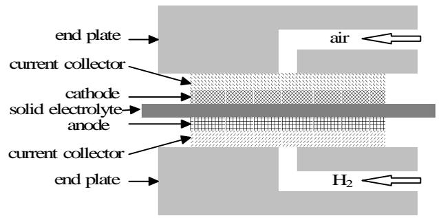
Fig.1 Schematic of the experimental cell set up.
