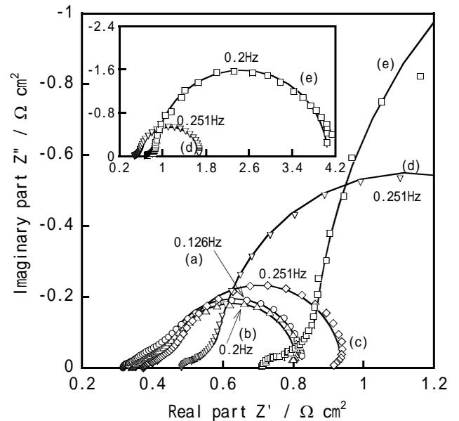
Fig.3 Experimentally obtained complex impedance plot of SOFC(56.8cm<sup>2</sup>) with various fuel utilization under constant fuel gas flow rate at 1023K.
