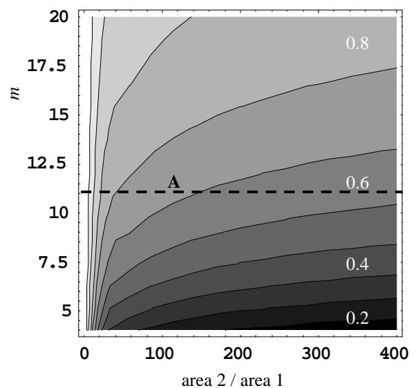
Fig.3. Effect of the Weibull modulus,  $m$  and ratio of cell component size (2) to tested specimen area (1) on the MOR. The strength reduction curves are plotted.
