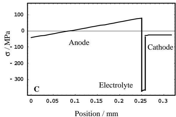
Fig.2. Example of the residual stresses in a SOFC cell (variant C).
