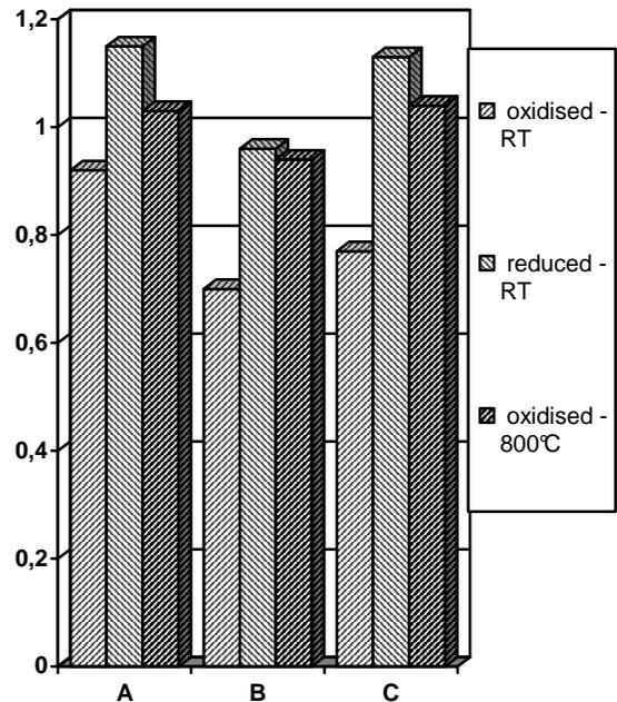
Fig.1. Normalised experimental fracture loads for variants A - C. Shown is a comparison of results for anode in tension to electrolyte in tension.
